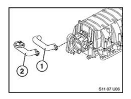
2. 2. Remove and discard the ventilation hose (1). Install the modified insulated hose with the external pressure regulating valve (2), using P/N 11 61 7 563 476 in the same location.
