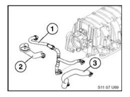
2. Remove the crankcase ventilation plastic corrugated hose (1) connecting the two cylinder head covers and intake system. Install the modified insulated hose with the external pressure regulating valve (2), using P/N 11 61 7 563 476. Install the insulated hose (3), using P/N 11 61 7 547 186.
